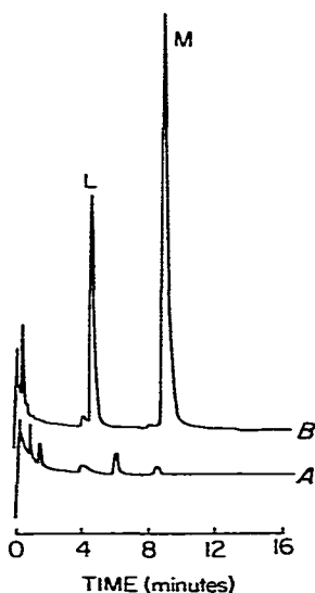
Fig. 2. Gas-liquid chromatograms of (A) extract of 1 ml plasma obtained from subject prior to receiving lidocaine and (B) 2 h after receiving 25 mg lidocaine hydrochloride intravenously. Peaks: L = lidocaine, M = mepivacaine (internal standard).
